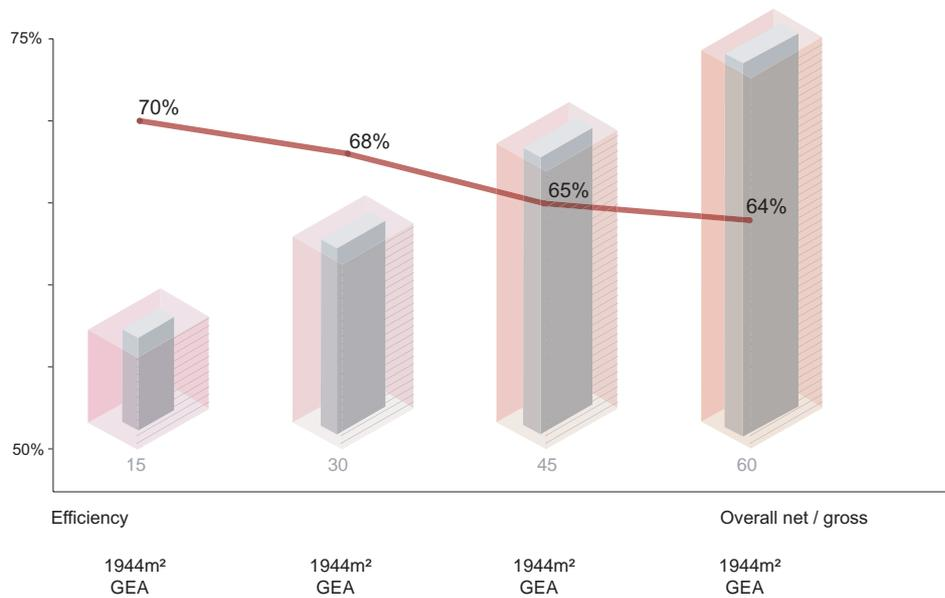
← Efficiency: the ratio of net to gross space – the building's efficiency – will decline with increased height. This reflects the larger core area required to serve a greater number of floors.
