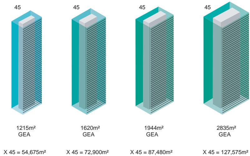
→ Cost Model Two: impact of size of the floor plate on the efficiency and cost of a 45 storey tower. © Davis Langdon LLP/KPF
