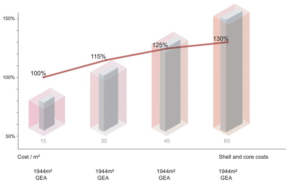
← Shell and core costs: shell and core cost per m<sup>2</sup> rise with buildings of increased height.
