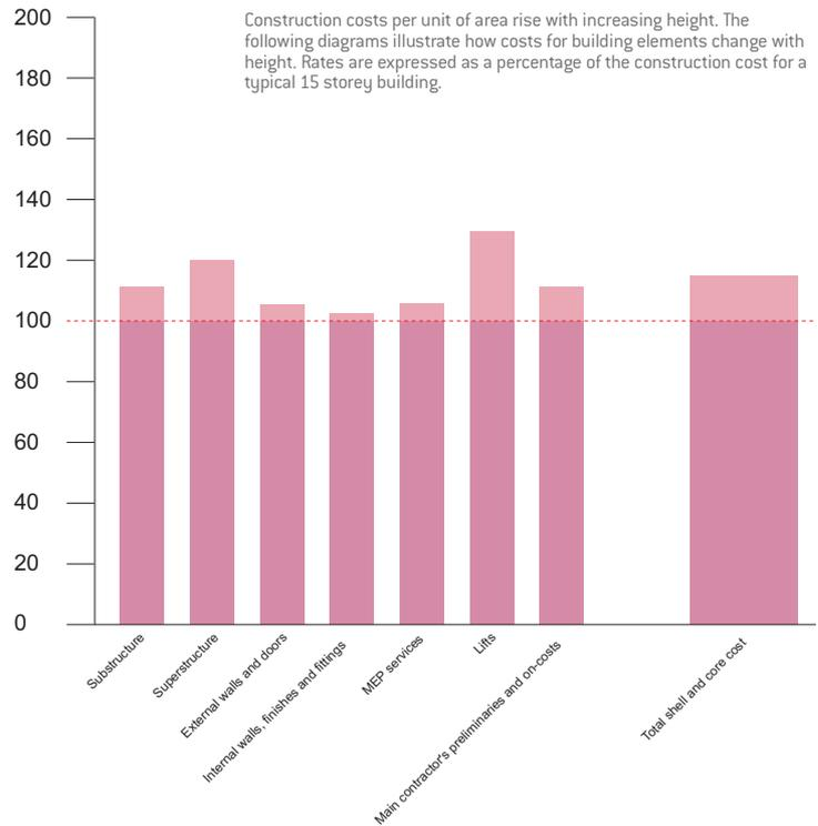
Construction costs per unit of area rise with increasing height. The following diagrams illustrate how costs for building elements change with height. Rates are expressed as a percentage of the construction cost for a typical 15 storey building.
